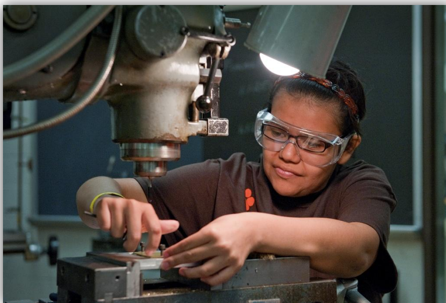
An EYF student operates a mill machine. The mill machine cuts metal into a specific shape, which then can be engraved later with the student's name.
