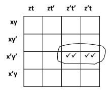
**Step 1**: Carefully draw the Karnaugh map, making sure the headings are exactly like those in the "setup" diagram.
