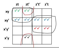
**Step 1**: Carefully draw the Karnaugh map. Note how the term x'y marks all squares beginning with x'y (highlighted in blue). These all like along the x'y row. Further note how the term xyz will mark all squares that begin with xyz (highlighted in green), and the term x'y'z' will mark all quares that begin with x'y'z' (highlighted in red).
