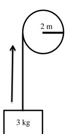
For one rotational revolution of the pulley, the distance the weight is raised is equal to one circumference; therefore,  $2\pi r = 2\pi \cdot 2 = 4\pi$ . The gravitational force on 3 kg is determined by  $mg = (3 kg) \cdot \left(9.8 \frac{m}{s^2}\right) = 29.4 N$ . Therefore,
