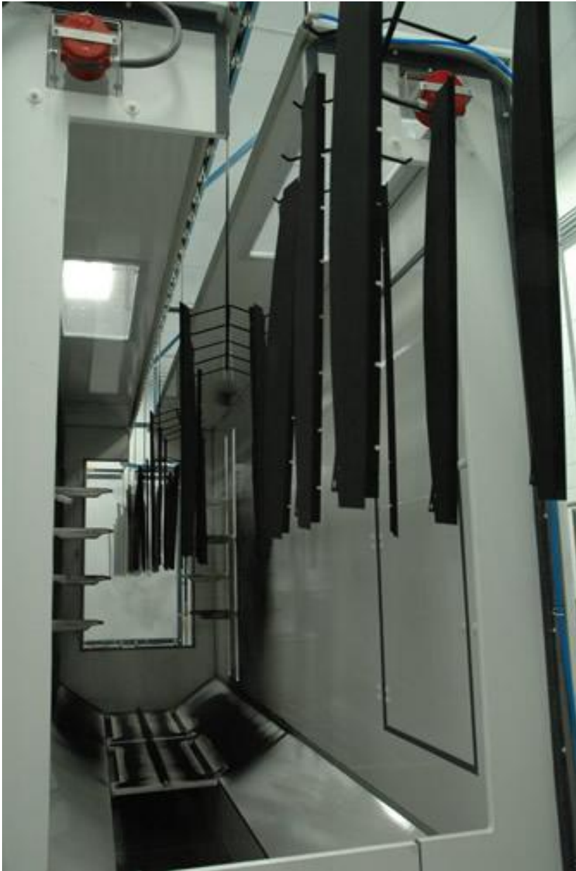
Example of a powder coating booth
