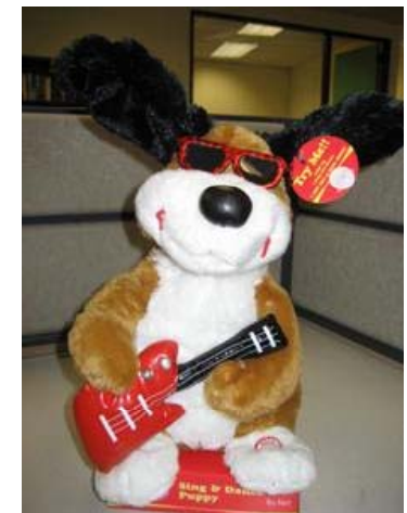
Red guitar 2,693ppm lead 34,775ppm chlorine 319ppm arsenic chromium, tin, antimony also detected
