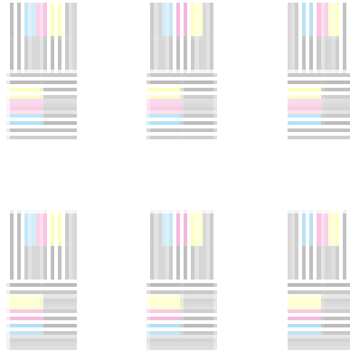
Figure 5. Color to Color Registration Test Target. IQAF CMYK Target Set, Xerox Co.
