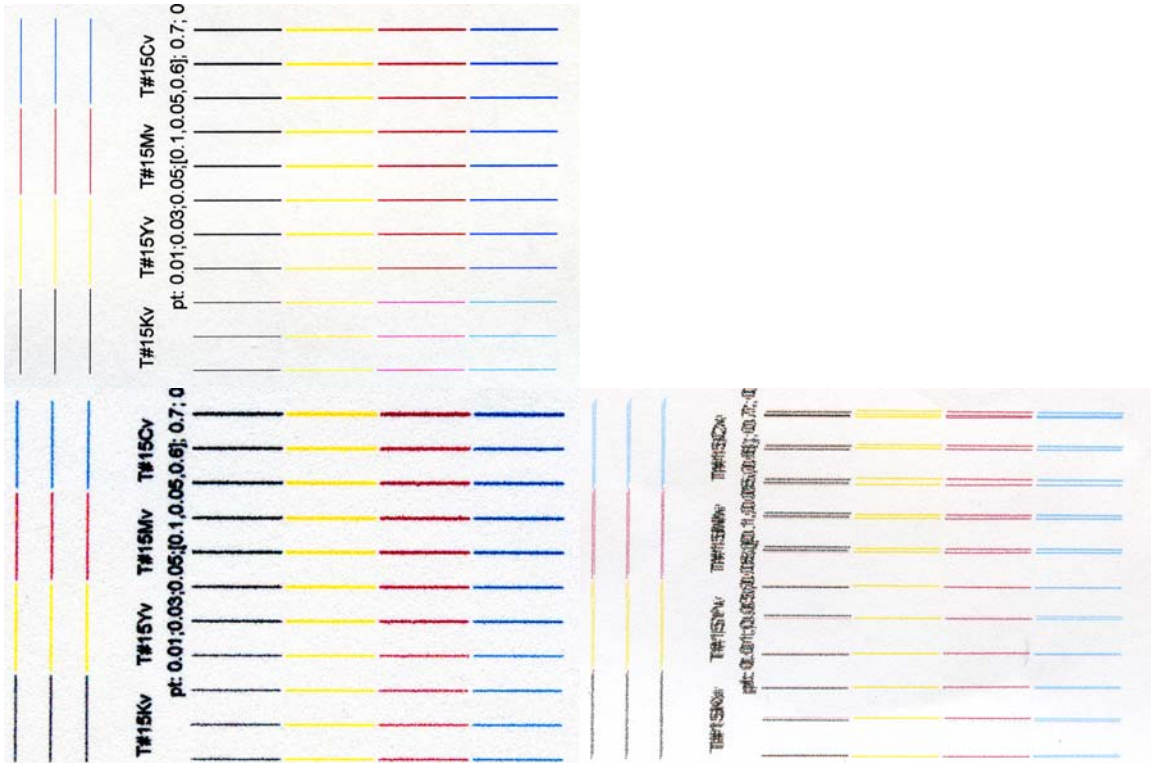
Figure 10. Fine Line Detail Test Target Scans. Top left image was printed by the Kodak EasyShare 5100 in 1G. The bottom left image is from the Epson R280 printer in 1G and the same printer produced the bottom right image in 0G.
