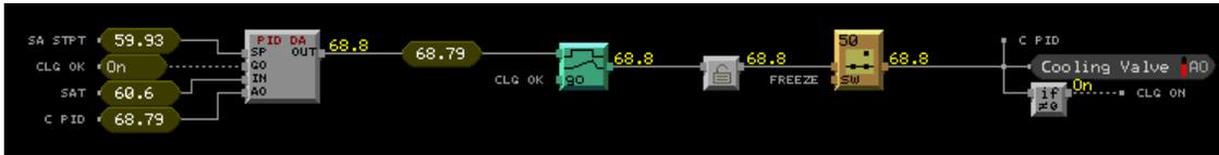
this example, notice how the final output is used as an input to the PID block. This output feedback is used to ensure that the PID does not deviate too far from the output when other parameters are affecting the output besides the PID block. These parameters might be a ramp block, limit block, or switches. Use this method whenever possible.
