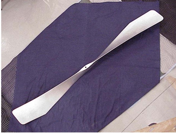
Figure 1 – 1911 Wright Bent End Propeller
