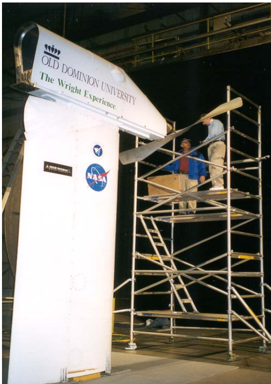
Figure 6 – Bent End Propeller Mounted for Test
