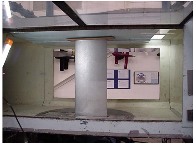
Figure 2 – Test Section Installed in Wind Tunnel
