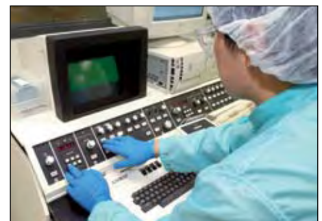
Top: A silicon wafer being prepared in RIT's Center for Nanolithography Research. Above: Jianming Zhou, a microsystems engineering graduate student, uses a scanning electron microscope to check 45 nanometer lines produced in the lab.
