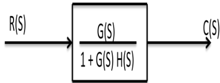
Figure 2: open loop representation of the Closed loop system of figure 1
