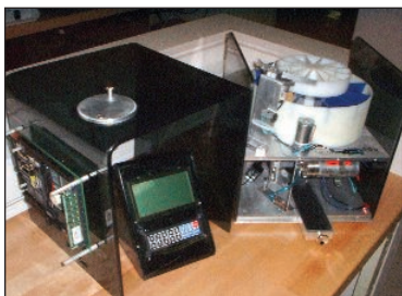
Working prototype of the Automated Home Medication Dispenser developed by RIT engineering students.
