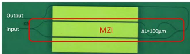
Fig. 5. Microscope image of the hybrid Si-LiNbO<sub>3</sub> modulator integrated into a Mach-Zehnder interferometer. The total size of the device is only 1 mm.
