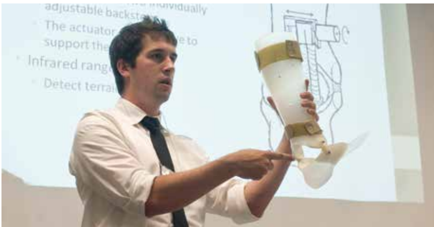
Improved Ankle Foot Orthotic (AFO): A common reason a patient is prescribed an AFO is a condition called foot-drop, a disorder involving a lack of ability to articulate the foot. Jointed plastic AFOs that hold a person’s foot in a neutral position are the current standard for addressing foot-drop. Interviews with patients and clinicians identified current AFOs need to allow for greater ranges of motion while walking on ramps or stairs. Christopher Sullivan, as part of a Senior Design Project in the Kate Gleason College of Engineering, developed a prototype AFO that will provide a variable support system for the foot that addresses those needs.
