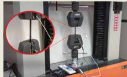
Electroactive Polymers (EAP): Gordon Goodman and the Lymphedema Engineering Group at RIT are researching the use of EAPs to make comfortable and expanding/contracting garments to address swelling. A sample is being tested for tensile strength in a stress gauge in order to characterize the material for further use.
