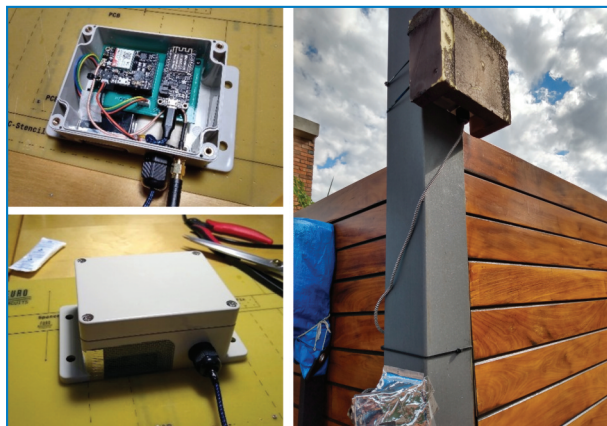
Figure 2. Sensor exterior and interior configurations with an example installation setup in Asunción containing a heat shield.
