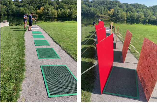
Fig. 1: Two of the four target setups. The left image shows the base setup of green sub-pixel targets with no shadowing or TR panels. The 20% target is closest in the FOV. The right image shows the TR panel and shadowing panel (TR-S) setup. The other two arrangements were the shadowing panel setup - which consisted of the shadowing panel from the right image without the bright red TR panel, and the TR panel setup, which consisted of just the TR panel. The color contamination from the TR panel may be seen on the shadowing panel in the right image.
