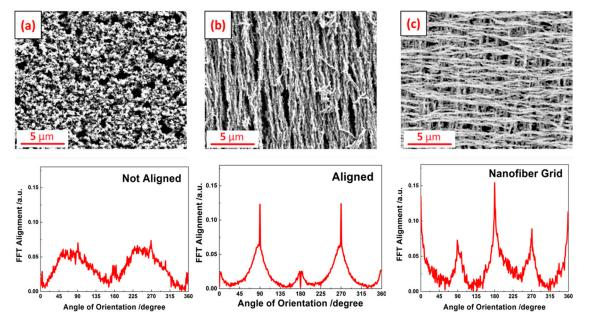
**Figure 6.** SEM images with corresponding 2D FFT alignment plots of two nickel layers sintered in (a) no magnetic field, (b) homogeneous magnetic field of 250 Oe in the same direction for all layers, and (c) multilayer printing and heating in presence of homogeneous magnetic field with alternating  $0^{\circ}$  and  $90^{\circ}$  orientations between layers.
