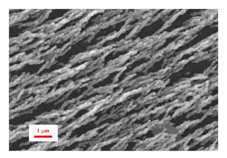
Figure 5. SEM image of aligned Ni nanowires (50% dilution).
