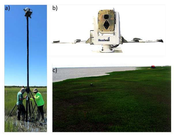
**Figure 2.** (a) Our HSI system being deployed in the field atop our BlueSky telescopic mast. (b) The different components of the HSI system. The Headwall hyperspectral sensor is housed within a maritime-rated General Dynamics Vector 20 pan-tilt unit. Our HSI system also incorporates a Vectornav VN-300 IMU-GPS to provide pointing information and GPS time-stamps. (c) A typical hyperspectral image obtained by our system on Hog Island at the VCR LTER.
