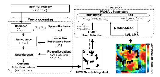
**Figure 4.** Overview of the inversion scheme to retrieve aboveground biomass of *Spartina alterniflora* from imagery collected by a ground-based HSI system. After data preprocessing, the NDVI threshold mask is used to remove soil pixels from the image in the analysis. EFAST provides band selection, while optimization of the PROSAIL model to obtain LAI and LMA uses the Nelder–Mead algorithm [77].
