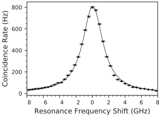
FIG. 2. The locations of the resonances for resonator two are scanned via resistive heating. We include a Lorentzian least-squares fit with a FWHM of 2.98 GHz. Each data point is collected with 3.0 min of integration.
