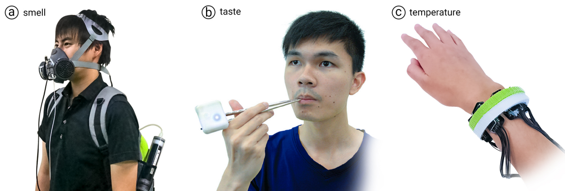
Figure 2: The Smell, Taste, and Temperature workshop covers chemo- and thermo-sensory interfaces. Above are three examples of such devices: (a) The Olfactory Assist Mask is a system that makes trace chemical gases interpretable to humans by substituting it with smellable odors [17]. (b) Ranasinghe et al. explored augmenting flavor by adding digital gustation to utensils like chopsticks [23]. (c) The ThermalBracelet is a device which provides fast-switching thermal feedback to the wrist using groups of four thermoelectric elements [21].
