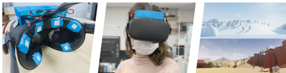
Fig. 1. Prototype of the ThermoQuest system worn by a user experiencing cold and hot immersive virtual environments.
