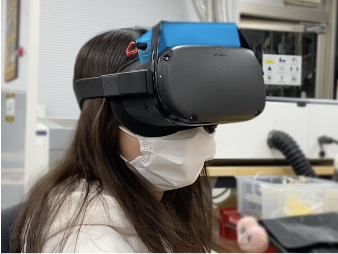
Fig. 4. User wearing the prototype of mobile head-mounted display with thermal feedback.
