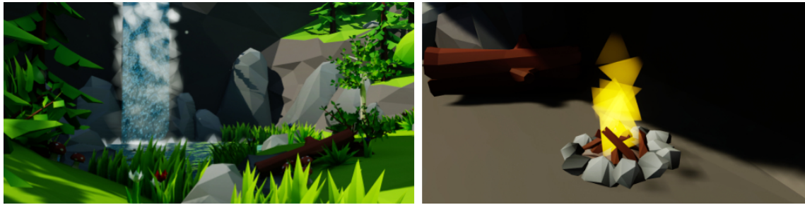
Fig. 3. Pictures from inside the VR environment showing thermally charged objects that generate cold and hot sensations. Proximity to the waterfall triggers cold feedback, while the fire produces heat.
