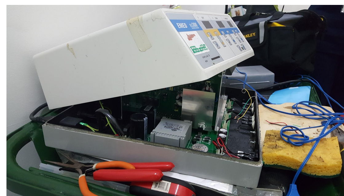
Figure 4: A damaged electrosurgical unit (ESU). This device required a complete replacement of the ground pad port.
