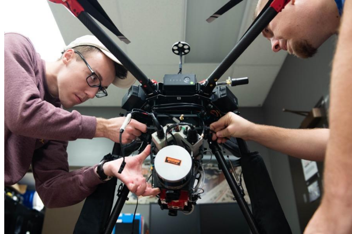
Imaging sensor package being integrated onto a UAV for precision agriculture studies
