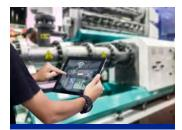
Machine monitoring encompasses hardware to collect machine data and software to analyze and display that data. It can be applied to critical production equipment and infrastructure systems. Machine monitoring is a key shopfloor application of the Industrial Internet of Things (IIoT).
