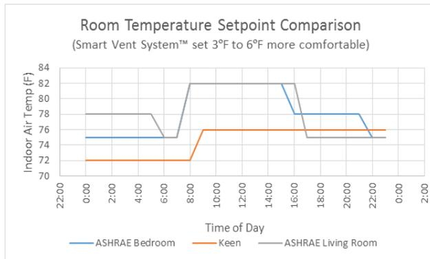
Comparison of ASHRAE recommended set points and the test house set points used during the project testing (Keen TX).
