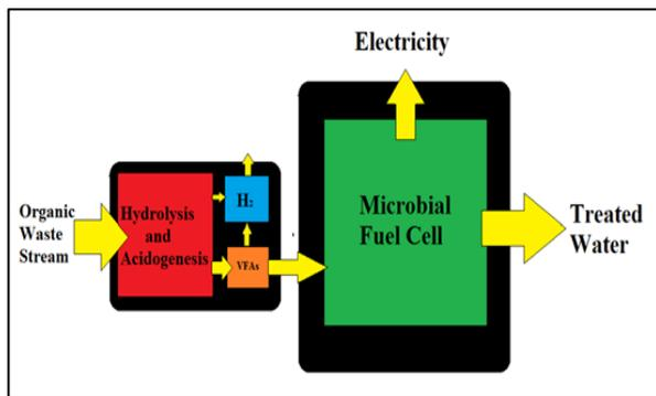
Pretreatment of glucose using a hydrolysis and fermentation bioreactor followed by a low pH microbial fuel cell resulted in a COD removal rate of 59mg/L-hr, which was almost a 5x increase over the glucose tests without hydrolysis.
