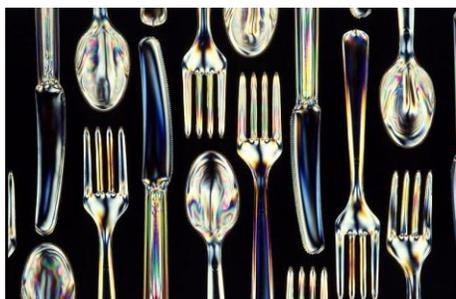
Flatware made from a biodegradable starch-polyester material. (Photo courtesy of USDA.)
