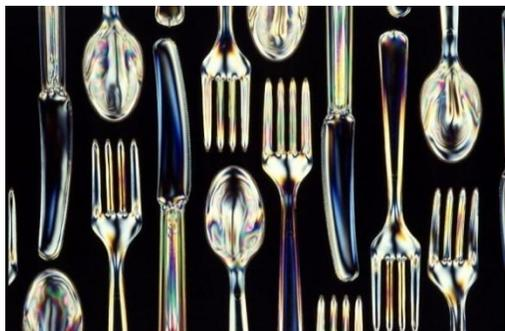
Flatware made from a biodegradable starch-polyester material. (Photo by USDA.)
