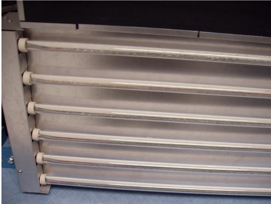
Example of typical quartz tube IR panel with ceramic fiber reflectors
