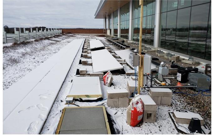
*Pictured: Comparative performance testing in progress on the green roof at RIT's Golisano Institute for Sustainability.*
