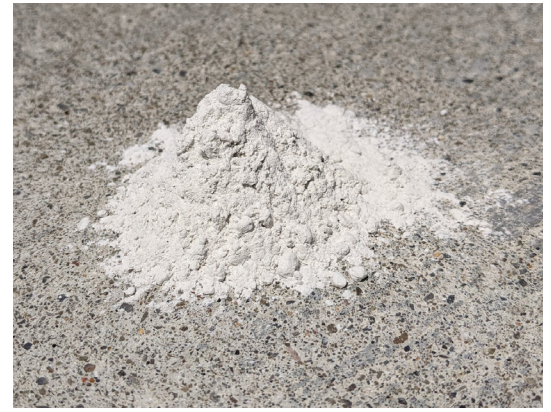
Pantheon™ is a partial cement replacement for concrete created from post-consumer glass.
