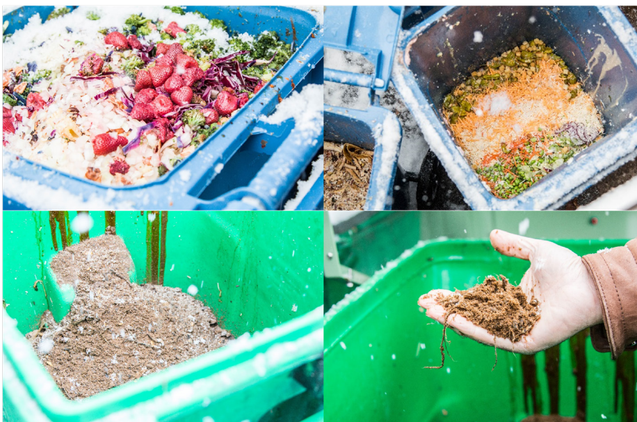
Examples of raw food waste inputs (top) and dried outputs from the WasteMaster (bottom)
