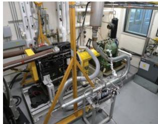
The goal of this project was to evaluate the performance of Paradigm's "Reactor" in the exhaust stream of a medium duty diesel engine by measuring exhaust gas emissions with and without the reactor present.
