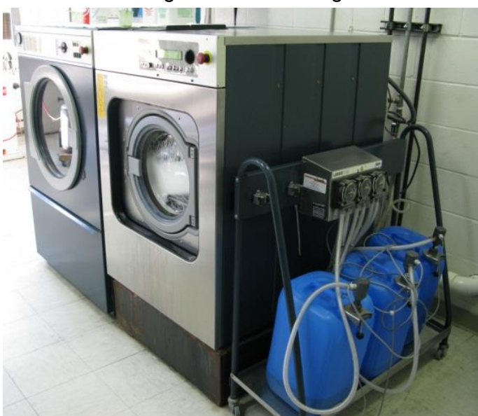
Figure 1. Typical wet cleaning dryer, washer, and detergent injection system (left to right)
