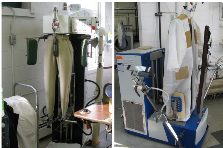
Figure 2. Typical pant topper (left) and form finisher (right)
