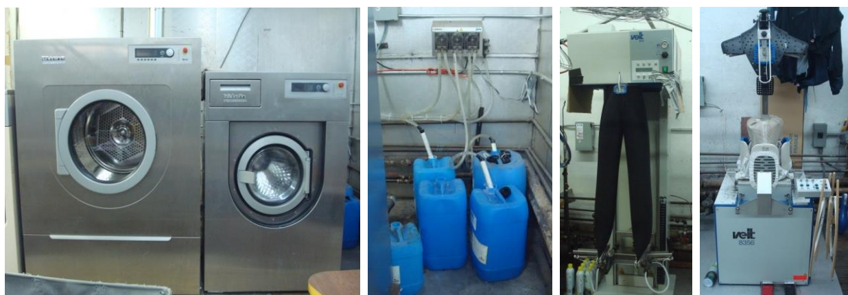
Figure 3. PWC system at a NYS cleaner, from left: washer & dryer, detergent injection system, pant topper, form finisher.
