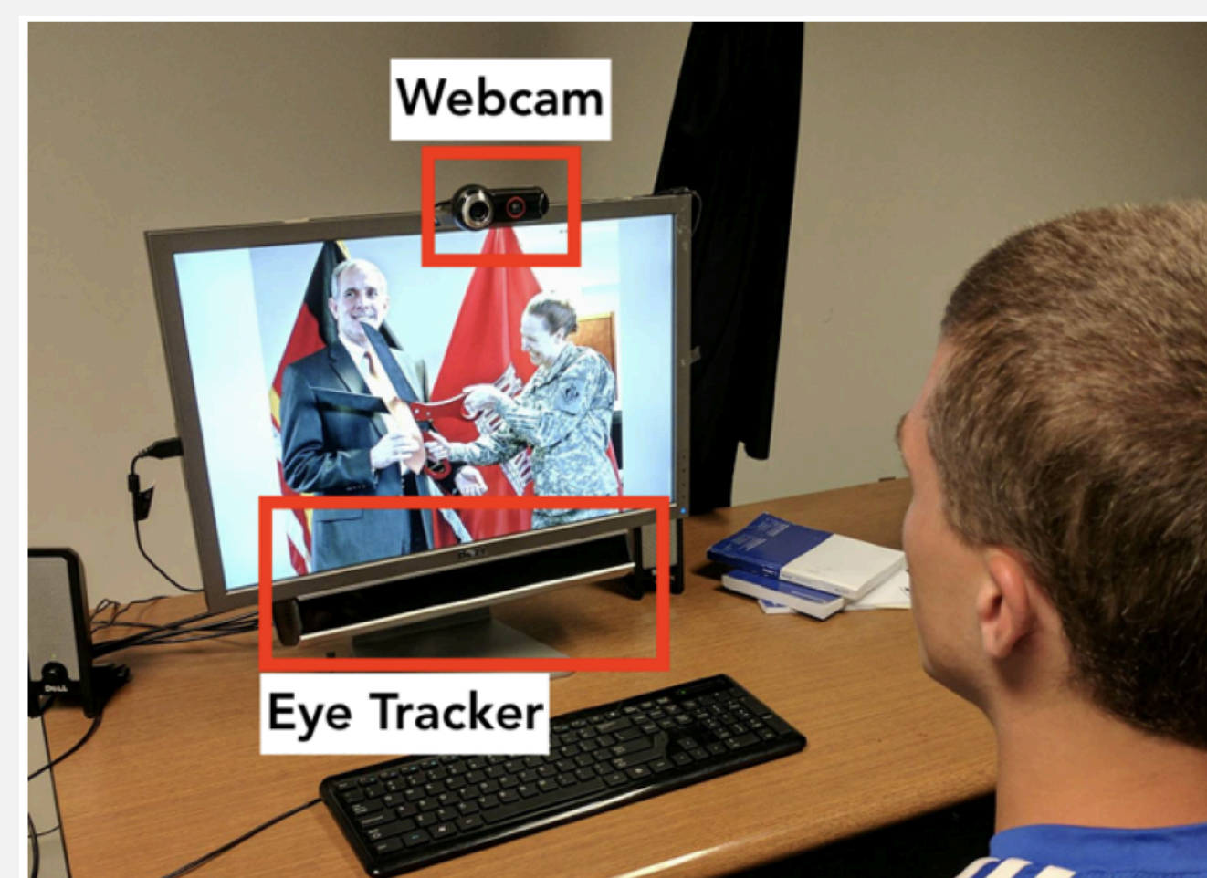
Figure 6: Observer in front of monitor with webcam and eye tracker. Lapel microphone used to record voice.
