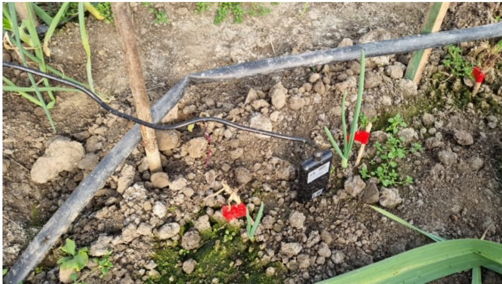
Figure 1: Integrated sensor for measuring soil temperature, pH level, light intensity, and nutrient levels (nitrogen, phosphorus, and potassium) deployed in the soil in the greenhouse of the partnering small family farm.
