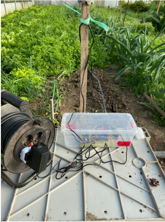
Figure 2: Setup of the connected ESP-32 board with WiFi module deployed in the soil in the greenhouse of the partnering small family farm.
