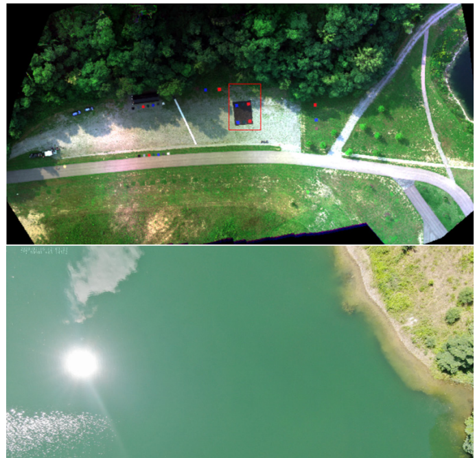
(top) Mosaic from the 5 band Micasense camera over our new Tait Preserve test area illustrating shadowing experiments and (bottom) a single image frame from an oblique RGB mission showing many sources of confusers (e.g., water glint, direct sun reflection, and cloud reflection).
