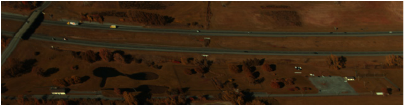
Figure. 1 A false color visualization of a hyperspectral frame of low-rate video of a highway scene. By flying along a highway, the vehicles moving in the same direction as the aircraft could be tracked for multiple frames. This oblique view provides tracking challenges due to shadows and obscurations.
