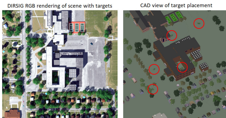
Figure 1: Example CAD view (right) of Megascene1 with T-72 tank targets placed in the open, along a tree-line, within an urban canyon, and next to a building side.
