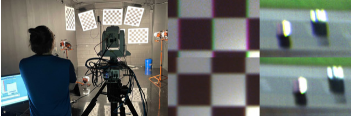
Figure. 2 Illustration of the spectral misregistration correction data collection procedure. The left side of the image shows the Headwall camera pointed toward a series of checkerboard targets. The top center and right images illustrate chromatic aberration at the edges of patterns, while the bottom center and right images demonstrates compensation for the chromatic aberration and thus much greater spectral fidelity.
