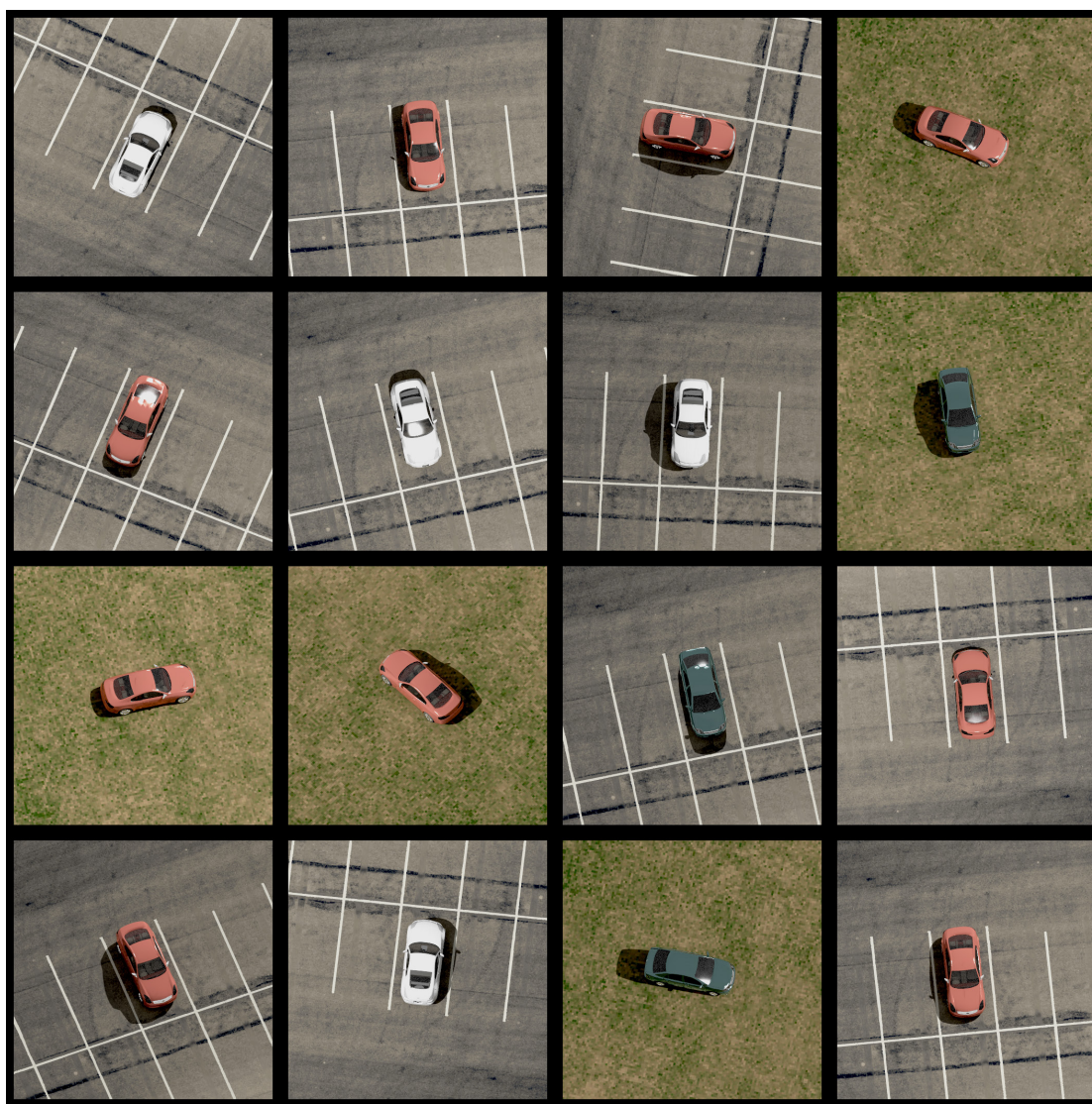
Figure 1: Output from a new capability within the ChipMaker plug-in for DIRSIG. Inputs include three targets (white Nissan Fairlady, red Nissan Infinity, green Toyota Corolla) and two backgrounds (grass, parking lot). This new capability produces randomized pairings of targets and backgrounds while also randomizing standard ChipMaker parameters such as view/source angles.
