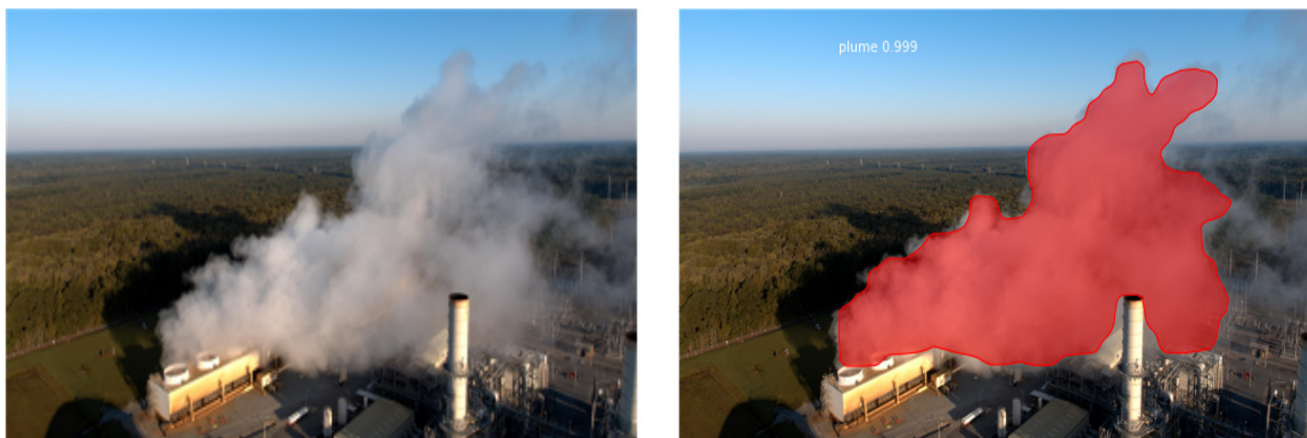
Figure 1: Trained Mask R-CNN model inference on imagery captured by drones at mechanical draft cooling tower test site.
