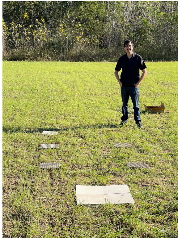
Figure 1: Imaging Science PhD student Chase Cañas observes a set of novel subpixel targets designed by him and deployed during a UAS collection at the RIT Tait Preserve in October 2021.
