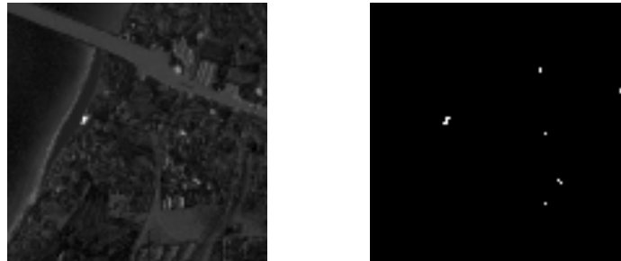
Figure 1. Result of hyperspectral target detection algorithm for tennis court spectra.
