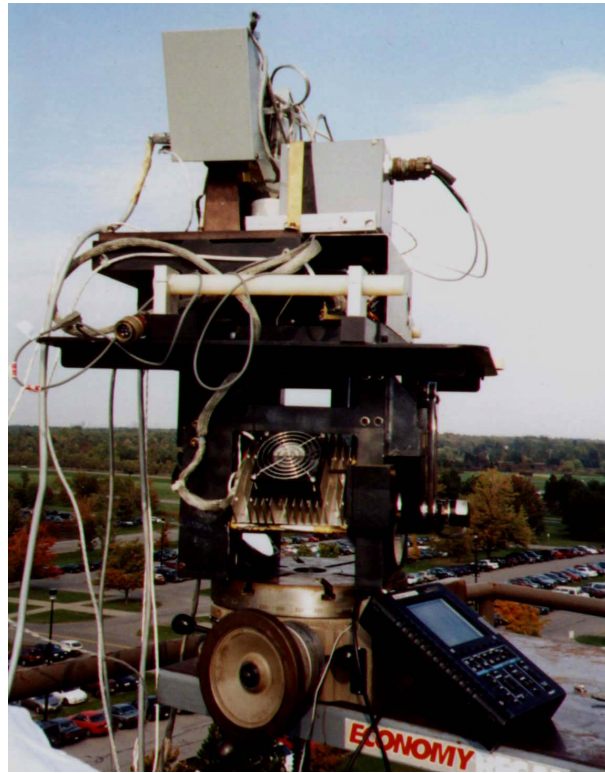
Figure 1 - MISI undergoing check-out and calibration on the RIT rooftop laboratory
