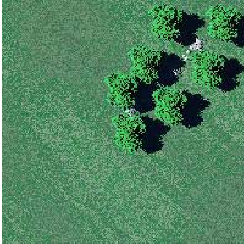
Figure 1: A true color DIRSIG scene containing a simulated grass fire. The fire pixels are the brighter pixels in the center of the trees. Spectral measurements of fire obtained at the Fire Sciences Laboratory were used to create the scene.
