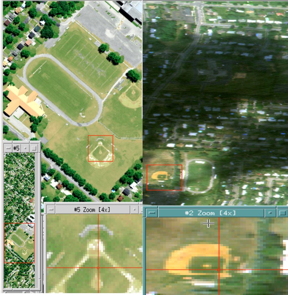
Visible color rendering of DIRSIG simulation of a section of MegaScene (left) and a MISI spectrometer image over another section of MegaScene (right). Both points highlight a corresponding grass pixel on a baseball diamond. Imaging parameters are slightly different and specified as follows (DIRSIG – HYDICE sensor; June 1, 2001; 1:00 PM local time; 2000 feet altitude; MLS atmosphere), (MISI – June 28, 2003; 12:35 PM local time; 3000 feet altitude; clouded atmosphere).
