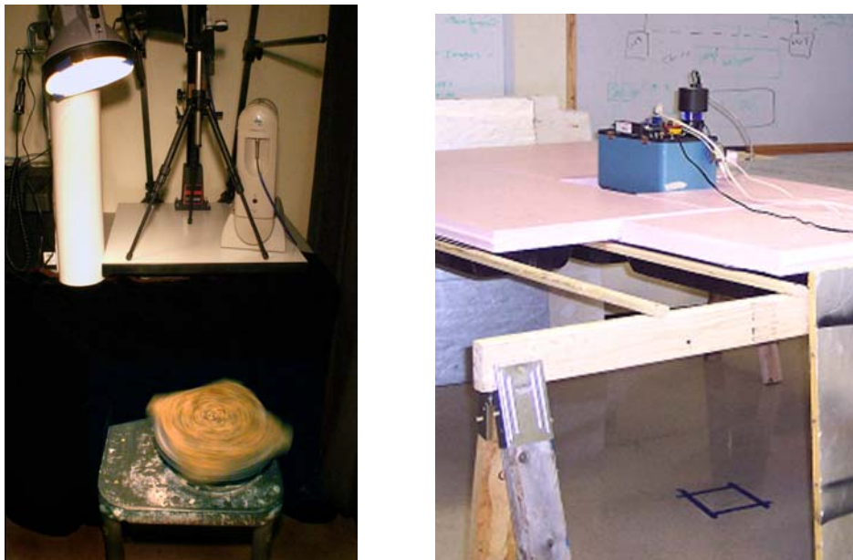
Figure 3.11.6-1: Laboratory set-ups for measuring spectral reflectance (left) and emissivity (right).
