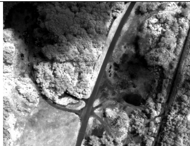
Figure 3.5.3-4c: Camera 1 with a NIR filter. The CIR filter is notched to allow spectral data above 714 nm to be captured and is used for monitoring chlorophyll bearing plants.
