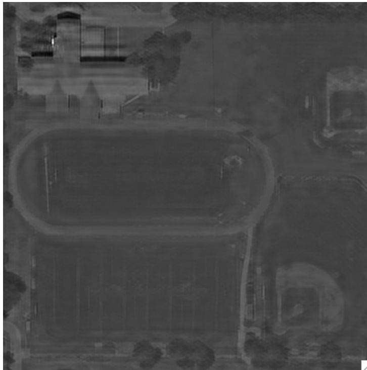
Figure 3.11.10-5: Object estimate based on the phase diversity algorithm of a triarm 9 sparse system shown in Figure 3.12.10-2.
