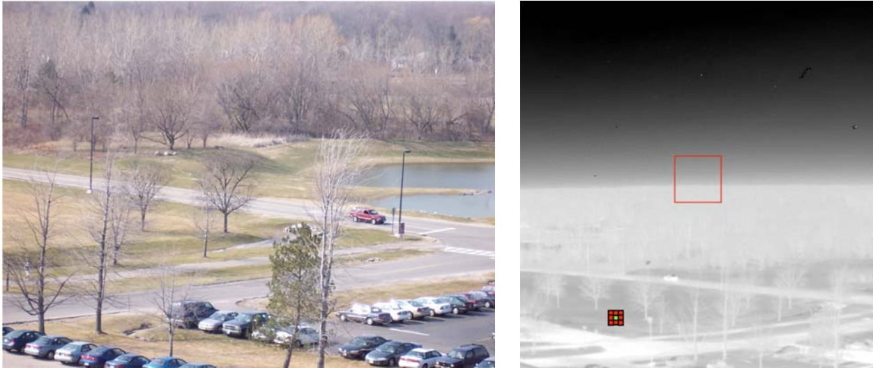
Figure 3.11.7-2: Thermal texture test scene imaged a) in the VIS with a handheld camera and b) in the LWIR by one of the cameras in the WASP sensor.
