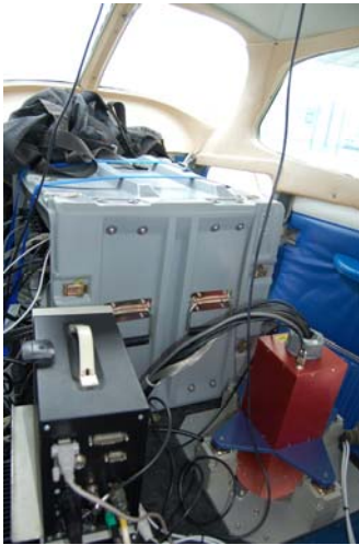
Figure 3.5.3-1: WASP-Lite in aircraft with filters attached and control electronics.
