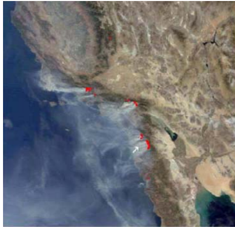
Figure 3.6-1: An image of the 2003 Southern California fires obtained with the NASA MODIS sensor. Pixels with active fire found using the statistical fire detection algorithm are marked in red.
