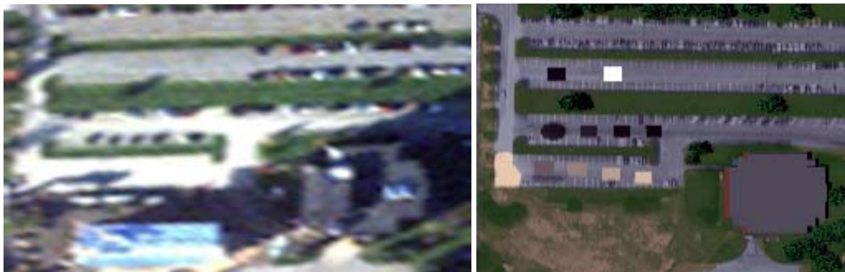
Figure 3.11.6-3: Airborne MISI image of sandy asphalt (left) and DIRSIG simulated image with varying amounts of sand and water on asphalt (right).
