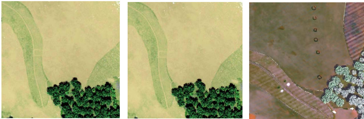
Figure 3.11.7-1: DIRSIG renderings of a portion of MegaScene 1 using (a) a single texture map, (b) three texture maps and (c) mixture maps.
