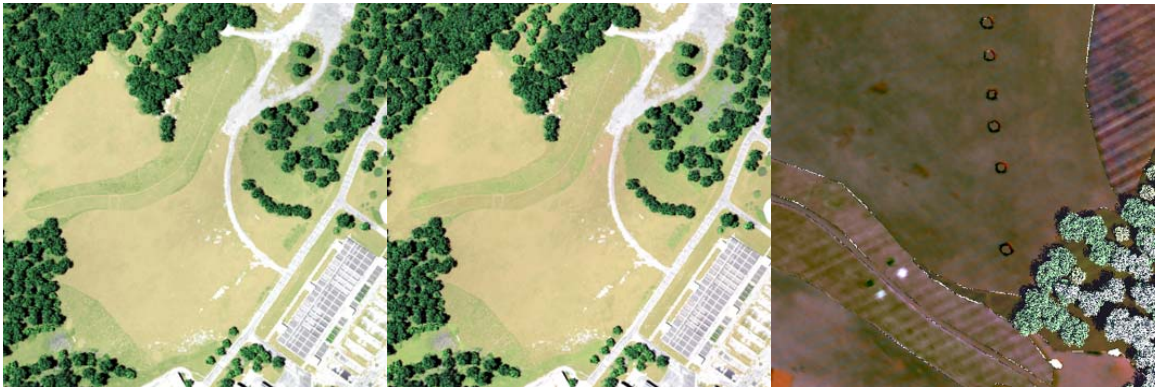
3.17.7-1: DIRSIG generated scenes showing texture results using the traditional single band approach, the multiband approach and (for a different set of conditions) the fractional mixing model approach.
