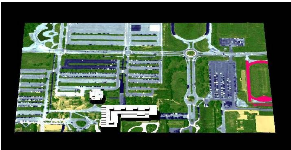
Figure 3.4.3-2: DIRSIG rendering of RIT campus derived from remotely sensed imagery and library databases.
