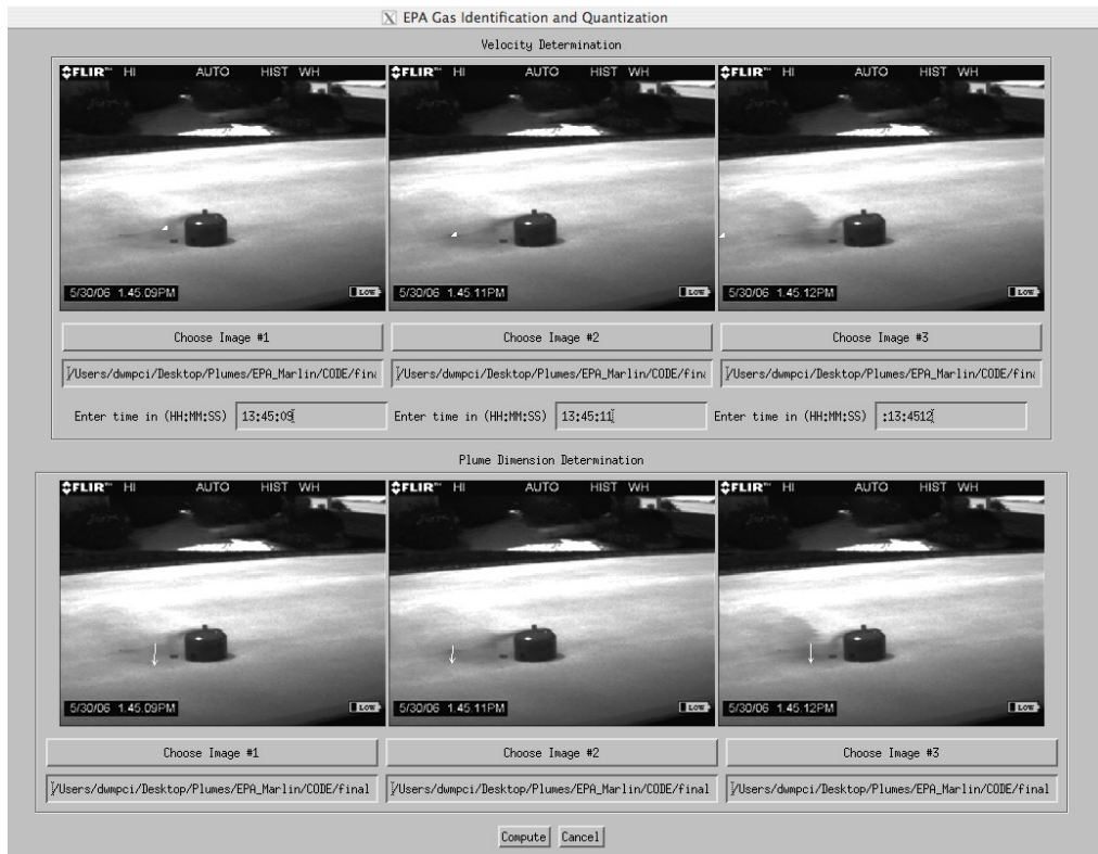
Figure 3.11.2-1: GUI in which the user interacts with the software to determine leak flow rate and size.
