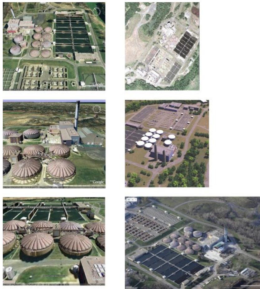
Figure 4.2-53: (left) Examples of actual imagery projected onto 3D wire frames of a site. (right) Two DIRSIG images of the site and a real oblique airborne image.
