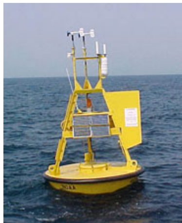
Figure 3.4-8: Picture of a NOAA buoy of the type deployed in the Great Lakes that records hourly air and water temperatures.
