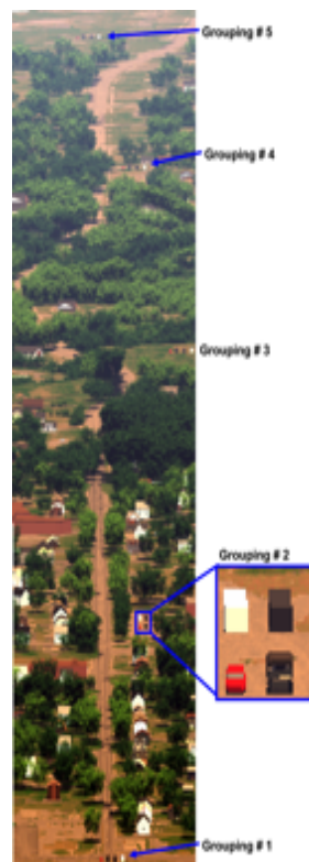
Figure 3.14-20: RGB image of DIRSIG hyperspectral oblique target detection scene with embedded targets.
