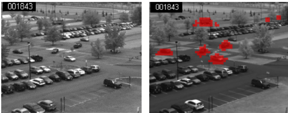
Figure 3.24-37: Motion detection at the pixel level for multispectral images collected from the roof of the CIS building. Red pixels in the right hand image are detected as moving in the time window considered (7 frames).
