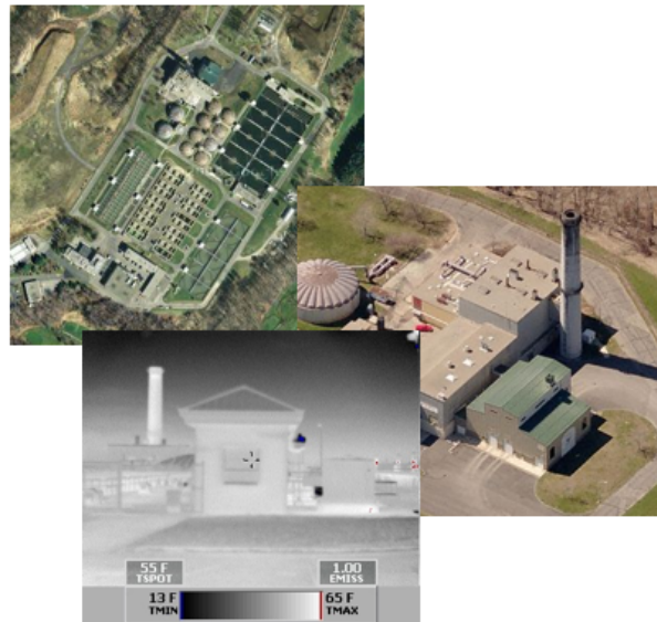
Figure 4.2-51: View of site from vertical multispectral sensor, oblique sensor and ground based long wave infrared sensor.
