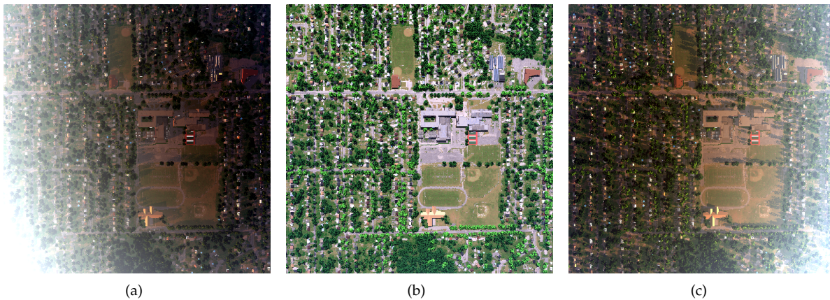
Figure 4.1-48: An image sequence of MegaScene #1 from a stationary camera acquired at (a) dawn, (b) midday and (c) dusk demonstrates the temporal aspects of the new run-time MODTRAN linkage with DIRSIG.
