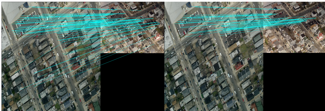
Figure 3.9-21: The top set of images shows matching between the two images using the SIFT matching process. The bottom set of images shows the matching after the outlying matches have been thrown out using the RANSAC process. (Images courtesy of Pictometry International Corporation).
