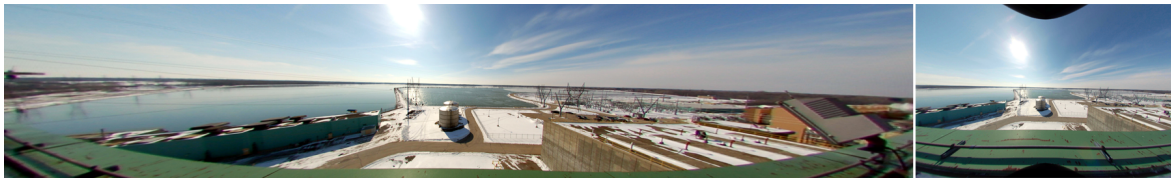
Figure 3.8-18: True color ground photograph collected with a Nikon D50 and a Sigma fisheye lens (left) of the MCV cooling pond from the plant roof. The geometric distortions were removed from this image producing the "defished" image on the right which was used to determine percent ice coverage on the lake.
