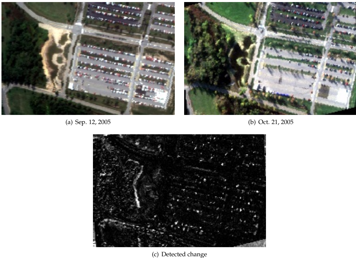
Figure 3.17-36: (a & b) Two images of the RIT campus collected with the MISI sensor, downsampled to the Worldview-2 spectral response. (c) The result of applying the Subpixel Hyperbolic Anomalous Change Detection tool to the two MS images.
