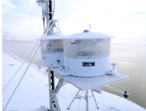
Figure 3.8-19: Eppley pyranometer and pyrgeometer that make up part of the shore-based weather station used on this ground collection campaign. The frigid conditions are obvious from ice layer that formed on the instrumentation.
