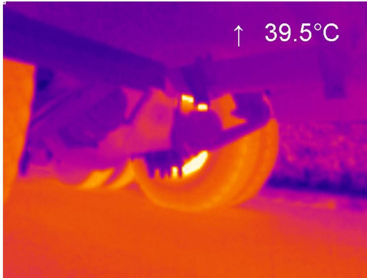
Figure 3.7-26: Rear drum brake on Ford F600 flatbed dump truck imaged by on-board MicroEpsilon thermal infrared bolometer camera during field experiment at the Wyoming County International Speedway.
