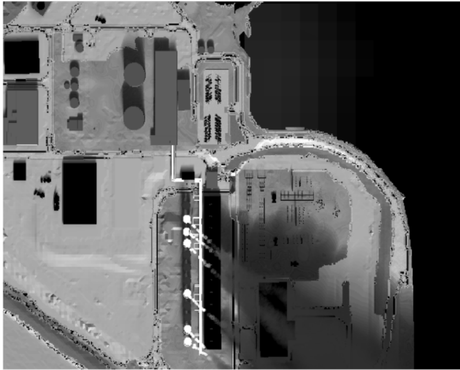
Figure 3.18-37: DIRSIG simulation of the Midland power plant as would be seen by an airborne LWIR system.
