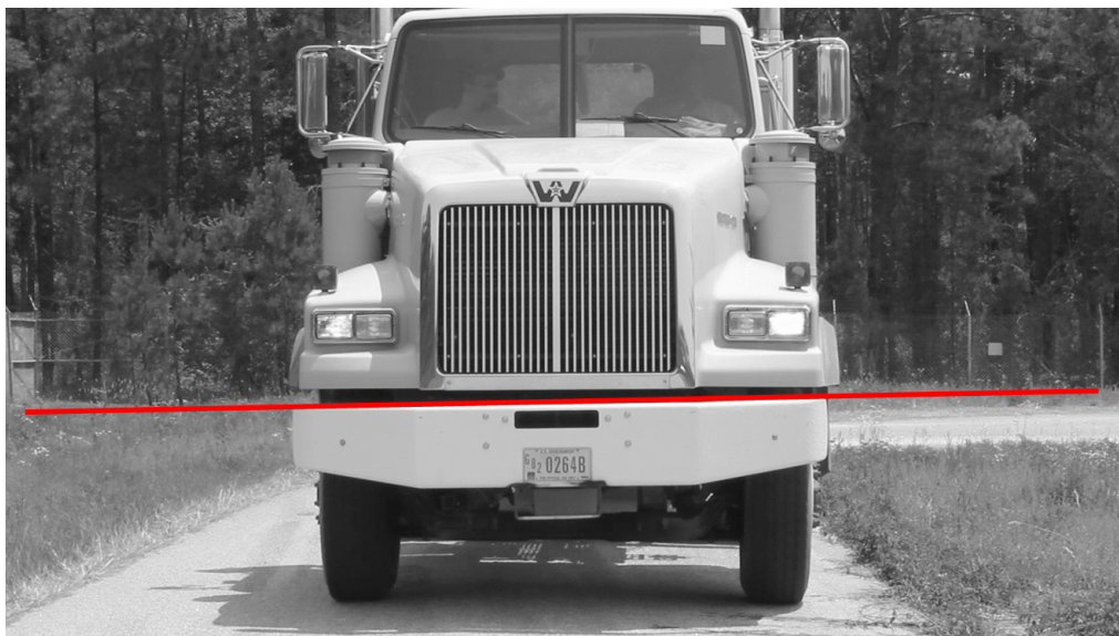
Figure 3.5-17: High definition video frame with the angle of the bumper being tracked to measure frame twist.
