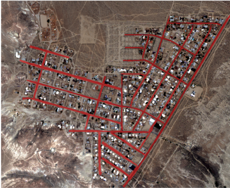
Figure 3.18-35: Results from processing a Worldview-2 multispectral image through the road network detection algorithm workflow. RGB image is shown with the detected road network highlighted in red.
