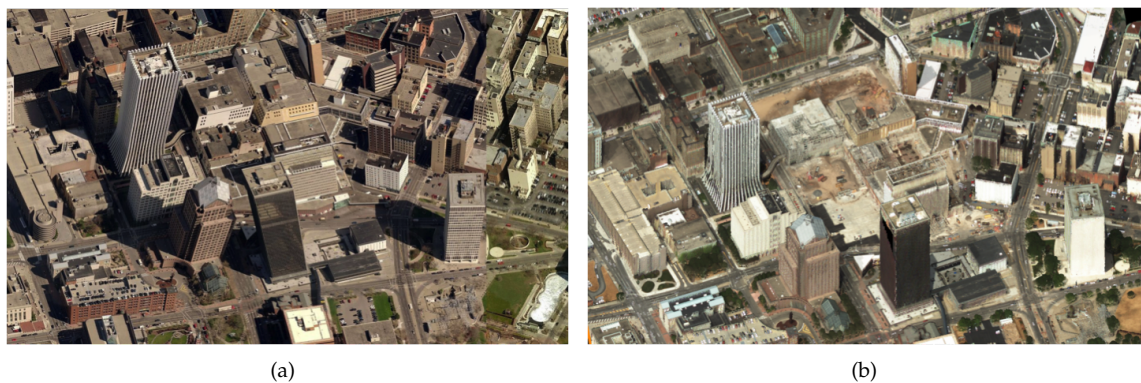
Figure 3.15-26: Comparison between traditional ortho photo and voxel-derived ortho photo. (a) Traditional ortho photo. (b) Ortho photo derived from projection onto the voxel model.
