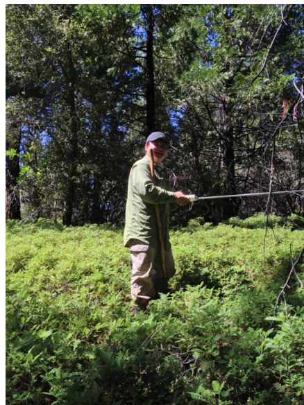
Figure 3.24-55: Graduate student Wei Yao (PhD) using an Accupar instrument to assess leaf area index (LAI) under a vegetation canopy at one of the field sites.
