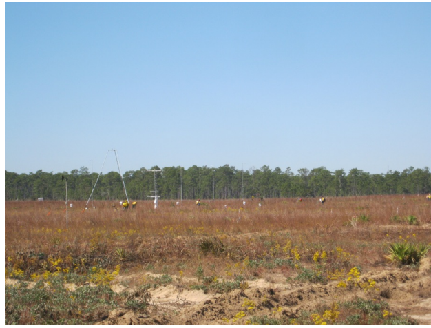
Figure 3.9-11: This picture shows the experimental layout of 25 RIT instrument towers deployed on one of the 10 ha 'small-series' fire behavior experiments on a grassland field at Eglin AFB, Florida. All the instruments here were RIT developed except for the tripod at the left-center of the photograph.
