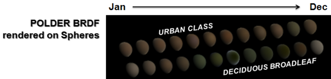
Figure 3.2-6: Example of the seasonal variation of polarimetric BRDF for two different land classes over the course of a full annual cycle derived from the POLDER BRDF database and rendered in DIRSIG.
