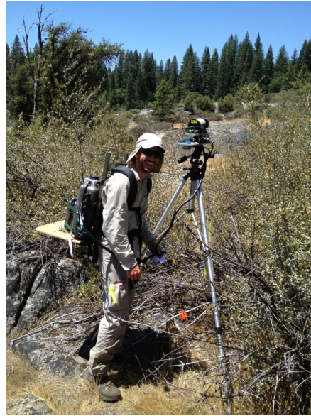
Figure 3.24-56: Dave Kelbe (PhD) using an in-house developed ground-based lidar system to collect detailed structural information for one of the study sites. Each lidar scans enables the team to construct a 3D representation of the surrounding area.
