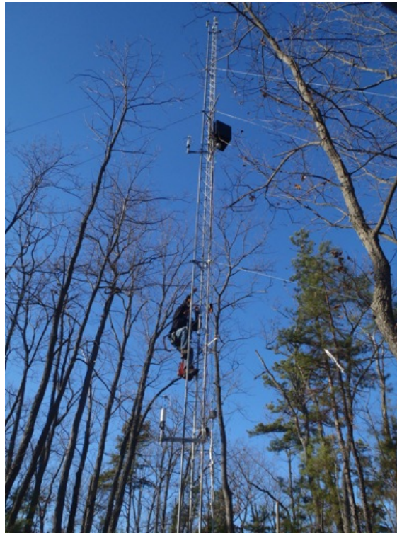
Figure 3.9-15: A 33 m meteorological tower measuring particulates and gas samples in and above the forest canopy. An RIT dual band radiometer was mounted at 8 m on this tower and also at 12 other locations on their own 6.7 m towers.
