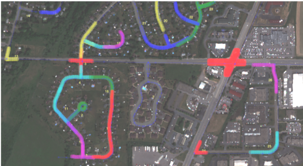
Figure 3.25-59: Image of a suburban area showing road sections and intersections identified in the image by leveraging Open Street Map data to prime a localized image search algorithm.
