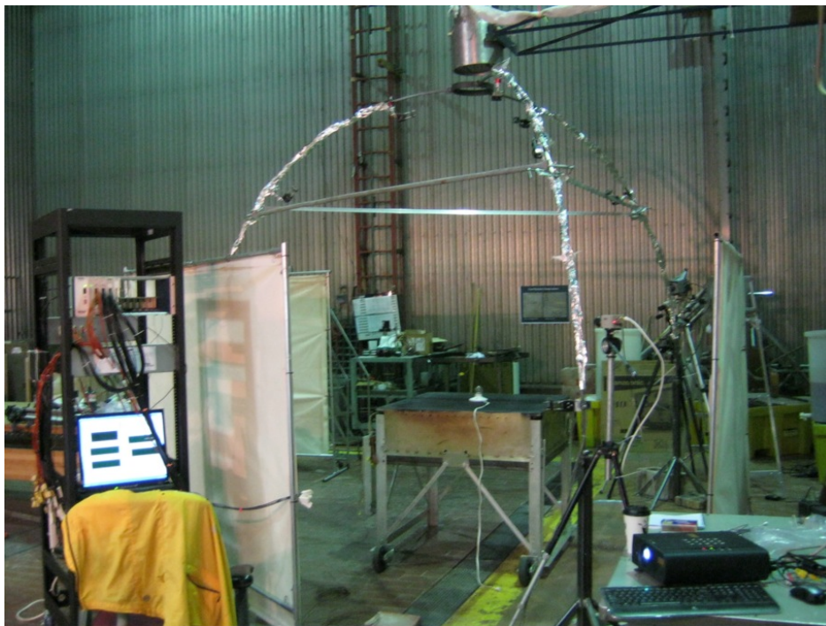
Figure 3.9-13: A photograph of the experimental set up in the main combustion chamber of the USDA FS Missoula Firelab. The semicircular bows support 9 narrow angle radiometers and other instruments used to monitor the symmetry of radiation form the fire.
