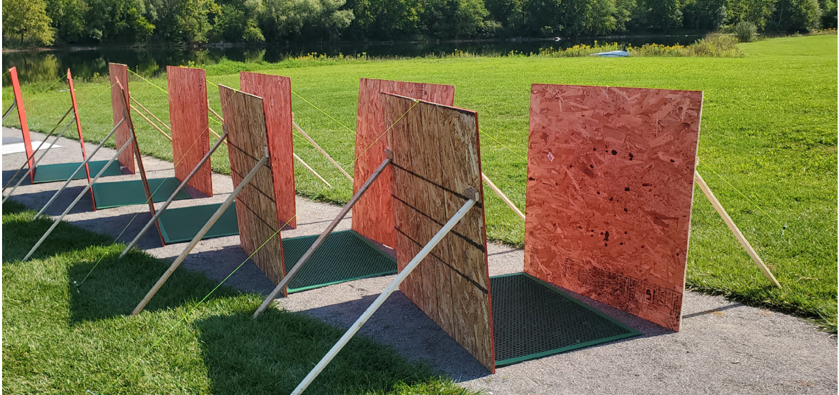
Figure 2: Novel subpixel detection targets deployed during September 2022 collection along with shadowing and reflector panels designed to explore nonlinear mixing effects in hyperspectral imagery.
