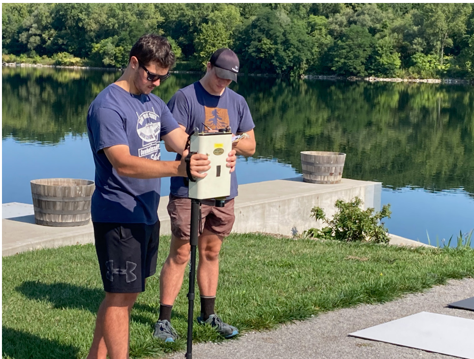
Figure 1: Imaging Science students Micah Ross (left) and Colin Maloney (right) collect ground truth reflectance spectra during a UAS collection at the RIT Tait Preserve in September 2022.
