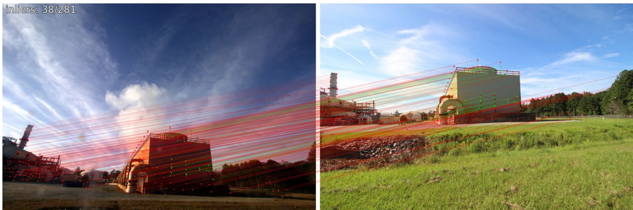
Figure 1: Query plume image with successful registration and (b) reference image with highest count of matched feature inliers tracked to the query image. Green lines show tracked feature inliers, where red designates outliers.
