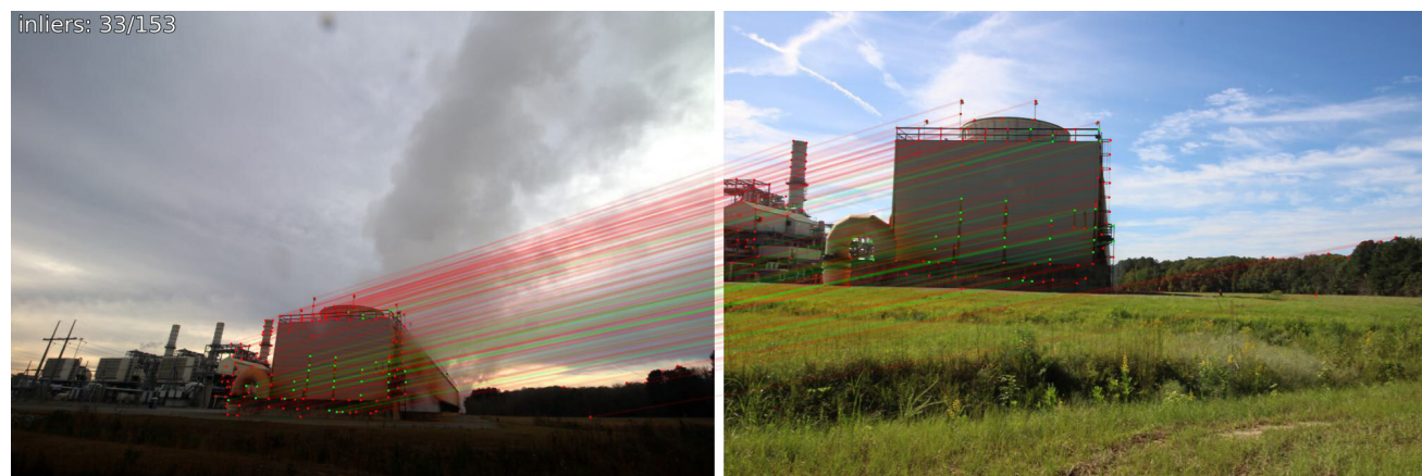
Figure 3: Query plume image with successful registration and (b) reference image with highest count of matched feature inliers tracked to the query image. Green lines show tracked feature inliers, where red designates outliers.
