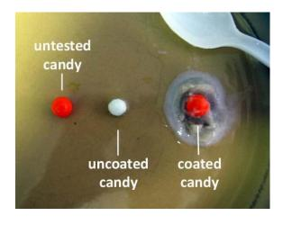
The image to the left shows what your experiment will look like after the candies have sat in the solution for about 8 minutes, showing us that the coating on the "pill" on the right delays the delivery of the drug in the stomach.
