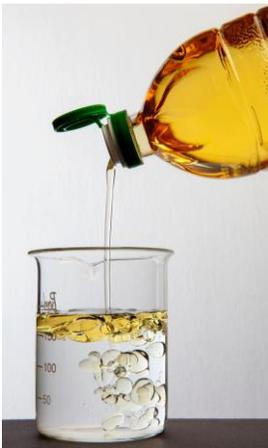
**Density** is a measure of how much matter occupies a given amount of space. We use the formula  $\rho = \frac{m}{V}$  to calculate density. The symbol  $\rho$ , pronounced rho, is used to describe the density of a mass ( $m$ ) divided by its volume ( $V$ ).
